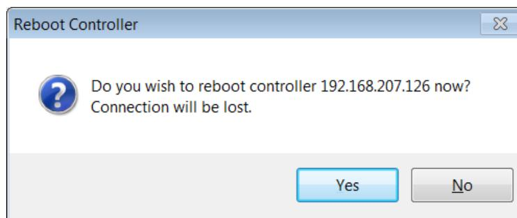
When the MP2600iec controller reboots, it performs a software reset on the ServoPack, so there is no need to physically remove power from the Servopack.
